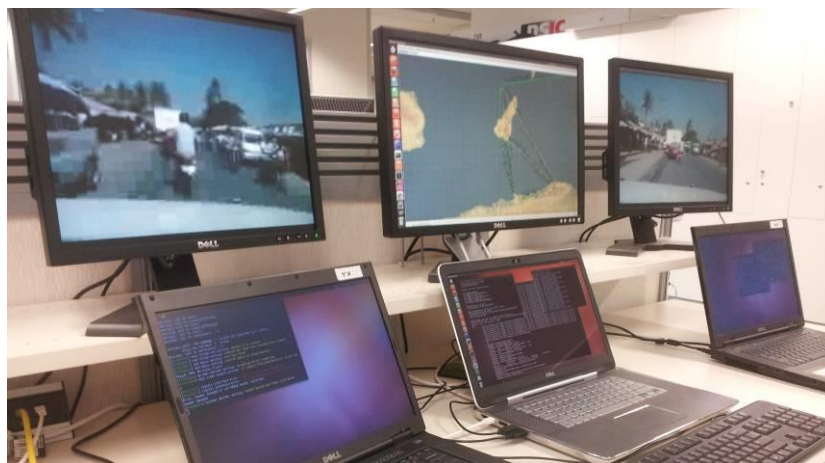
Figure 5: Experimental configuration, showing from left the transmitting PC (amphibious landing force), network emulation PC and receiving PC (remote base).
